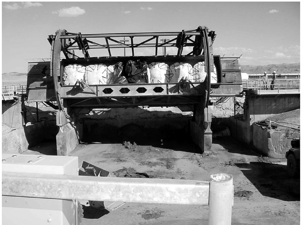
Figure 5: Rail Unloading Facility Associated with Class A Bulk Waste Disposal at the Envirocare Disposal Facility
